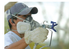
FTx 4-finger gun trigger – full length trigger is easier to hold in continuous spraying.
