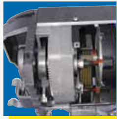
Toothed belt motor drive needs no maintenance .
